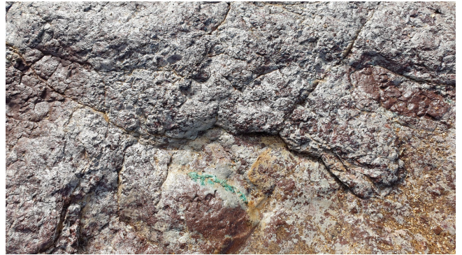
Copper ore Malachite appearing as green beads in lower centre of photograph
